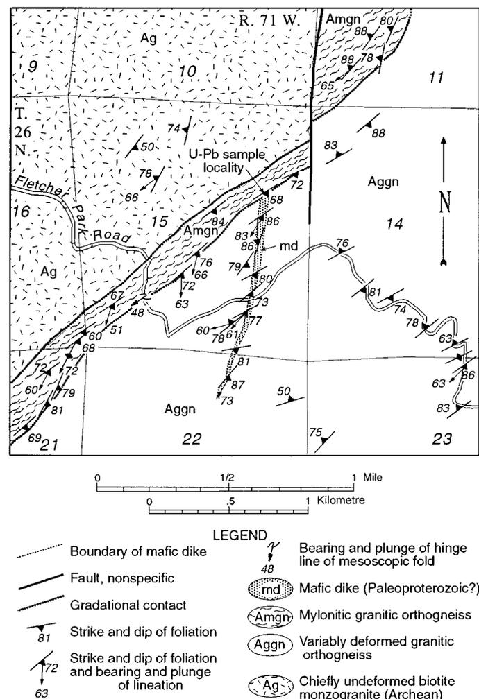
Figure 2. Geologic map of Fletcher Park area and mafic dike sample locality. Geology by A. W. Snoke (1993 and 1994). Only mafic dike that was dated with U-Pb techniques is shown. Area is widely intruded by mafic dikes of Paleoproterozoic age; distribution of these dikes is shown in Snyder et al. (1995).
