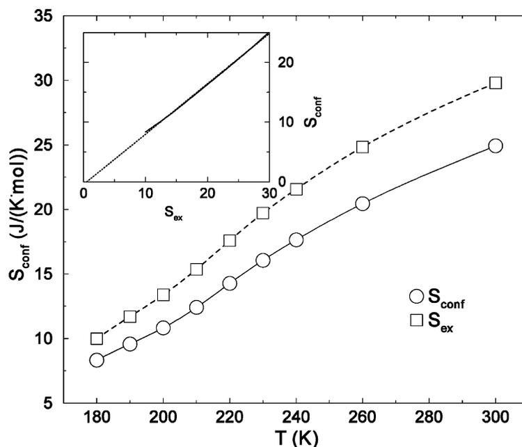
Fig. 2.  $S_{\text{conf}}$  and  $S_{\text{ex}}$  at a fixed density  $\rho=1.0 \text{ g/cm}^3$  for the SPC/E model. The inset shows a parametric plot (solid line) to demonstrate proportionality. Figure redrawn from Ref. [39].
