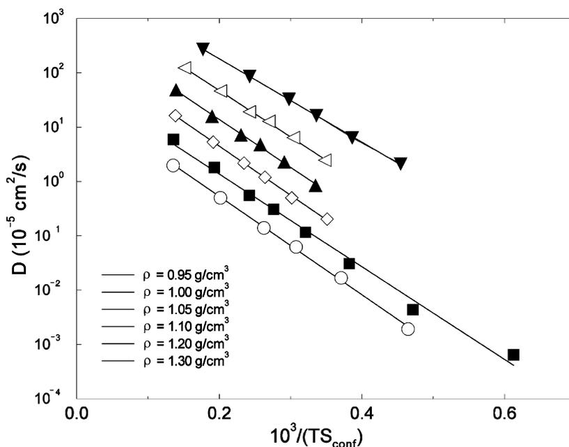
Fig. 1. The diffusion constant  $D$  as a function of  $1/TS_{\text{conf}}$  for the SPC/E model, confirming the predicted relation of Adam and Gibbs. Note that the curves for each density have been shifted for clarity. Figure redrawn from Ref. [35]. Verification of the proposed relation for simpler models is reported in Refs. [46–49].
