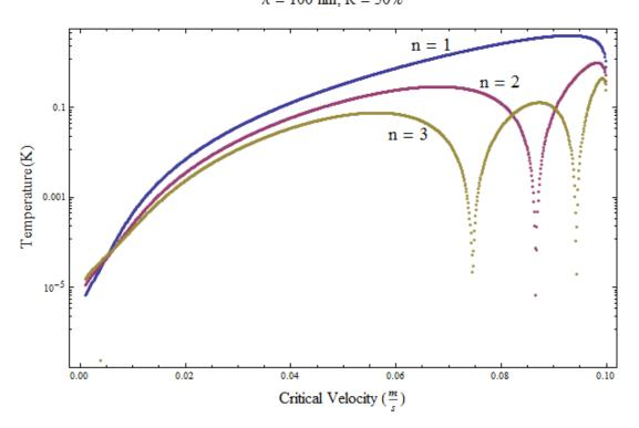
Figure 2.5 - Effective Temperature vs Critical Velocity plots with a reflection coefficient of 50%. Note: the discontinuities and decreasing values of the temperature in the Fourier modes are merely a result of resonance in the Fourier analysis, and do not represent physical phenomena.
