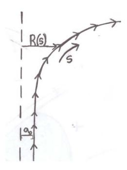
Figure B.2 - R(s) vs s for a given vortex core.
