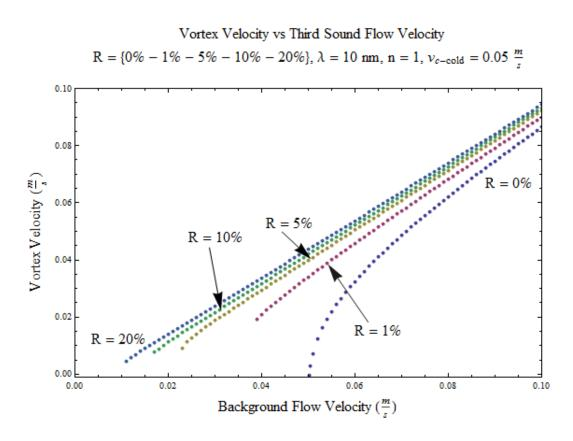
Figure 2.7 - Plot of vortex velocity  $(v_v)$  vs third sound flow velocity  $(v_s)$  for different values of the reflection coefficient.
