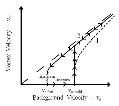
Figure 2.9 - Modified vortex dynamics. The vortex depins at  $v_{c-cold}$ , transfers to path 2, travels up path 2 to the peak of the third sound oscillation, then travels back down path 2, where it undergoes hysteretic motion when captured by the defect site at  $v_{c-hot}$ , and eventually repins. Paths 1 and 2 represent the static and dynamic drag paths, respectively.
