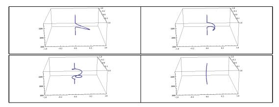
Figure 1.4 - Time propagation of Kelvin waves on a vortex core resulting from an initial Gaussian displacement. Propagation times are scaled to the core frequency. Top left: t = 0. Top right: t = 5. Bottom Left: t = 10. Bottom Right: t = 100.
