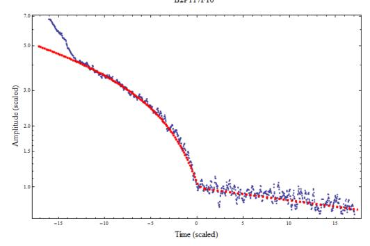
Figure 4.6 - Decay curve fit resulting from the dynamic drag model. Note a remarkably better ability to simultaneously match the curvature of the decay curve and the position of the critical point.
