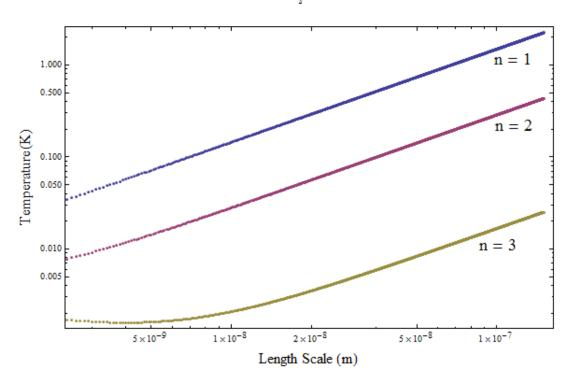
Figure 2.4 - Effective Temperature vs Length Scale ( $\lambda$ ) plots with a reflection coefficient of 50%.
