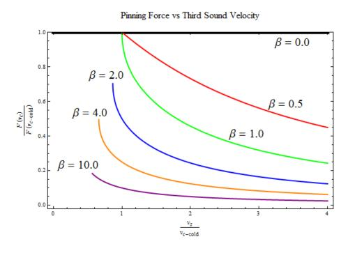
Figure 4.2 - Calculated scaled pinning force/critical velocity (Equation 4.4).
