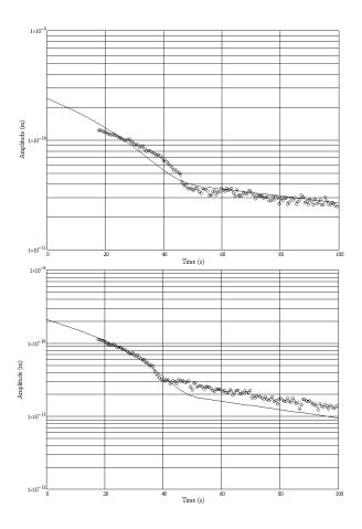
Figure 4.5 - Decay curve results from Anand Swaminathan's thesis [2]. There is an inability to simultaneously match the curvature of the decay amplitude and the critical point position.
