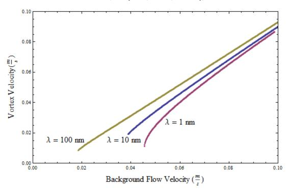
Figure 2.8 - Plot of vortex velocity  $(v_v)$  vs third sound flow velocity  $(v_s)$  for different values of the length scale  $\lambda$ .
