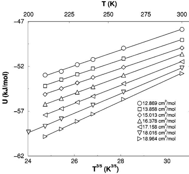
FIG. 1. Fit of the potential energy along isochores with the functional form  $U_0 + \alpha T^{3/5}$ . Symbols denote different molar volumes. For the sake of clarity, the different isochores are shifted by  $-1$  kJ/mol each in order to avoid overlaps.
