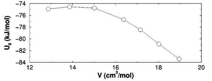
FIG. 2. Volume dependence of  $U_0(V)$  from Eq. (2). Note that this coincides with  $F(T=0 \text{ K}, V)$ . The negative curvature implies the presence of an unstable region in the phase diagram at low  $T$ .
